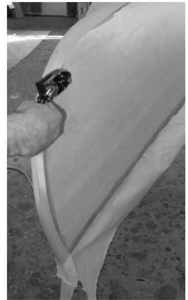
Figure 10. Using heat to activate the adhesive.
